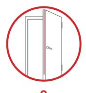
Check fire strips (usually a plastic strip with a fuzzy brush) are around the top and sides of the door or frame. Check they're intact with no signs of damage.
