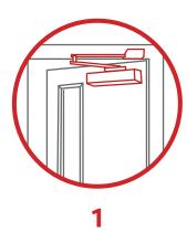
Check you have a self-closing device. The door should close firmly onto the latch without sticking to the floor or the frame.
