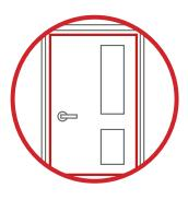
Check your door fully shuts into the frame and has no damage or holes. Open it six inches and make sure it can fully self-close.
